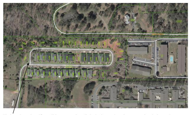
Hydrant Location. If possible you can install the hydrant where it was previously located.
